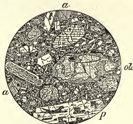
Fig. 33.—Basalt. Lion's Haunch, Arthur's Seat, Edinburgh. \times 8 . a , Augite. ol , Olivine, altering along cracks into pale green serpentine. p , Plagioclase, often corroded by the groundmass. Some magnetite. Hemicrystalline groundmass, in which the glass is much reduced by the abundant development of microlites of plagioclase and augite.
